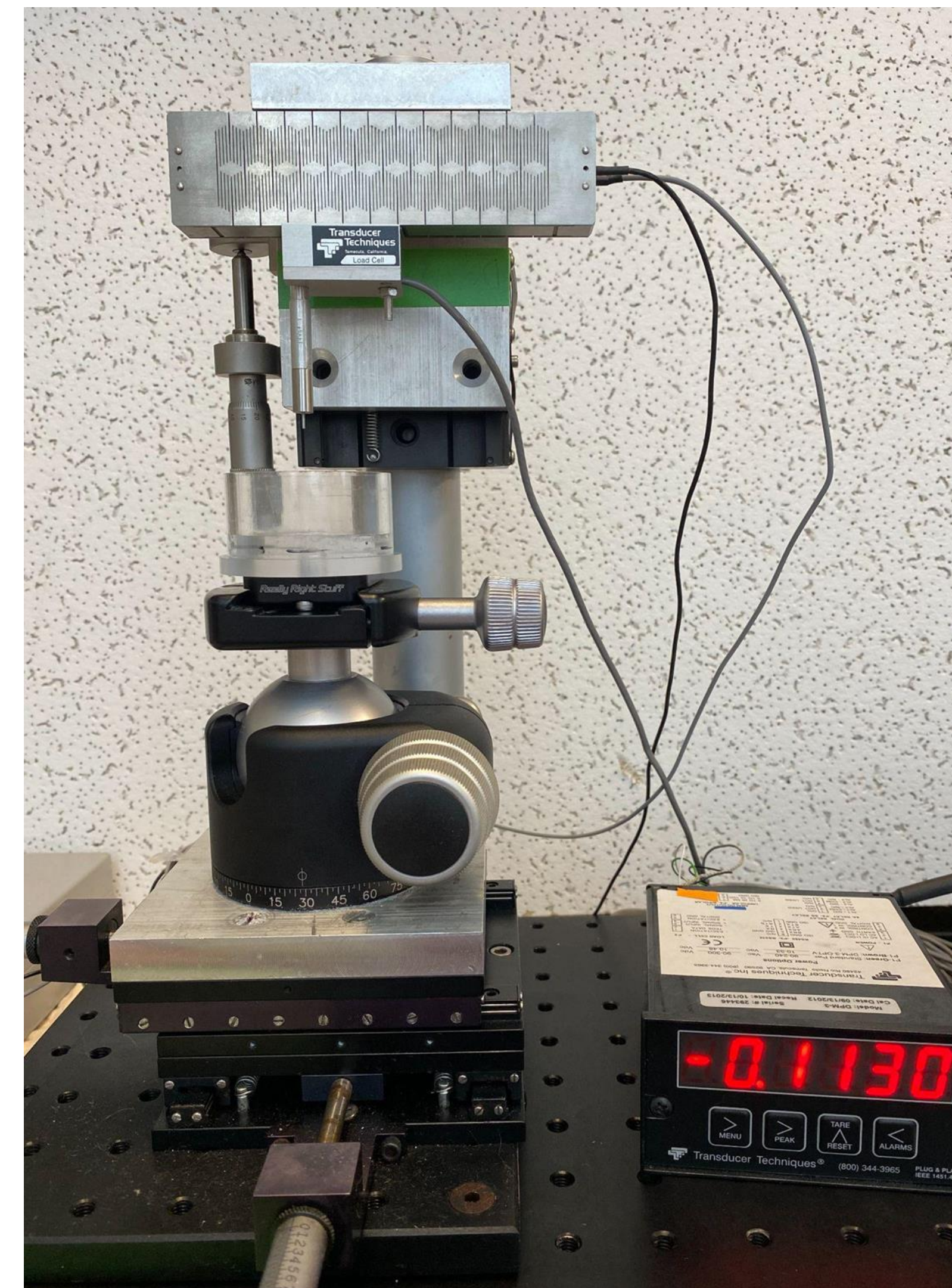
Fig. 3: Microindentation device after refurbishment. All hardware devices have been fixed and work properly. Software and code have been updated in a new computer, and successfully records all the data received, as seen to the right in Fig. 4.
